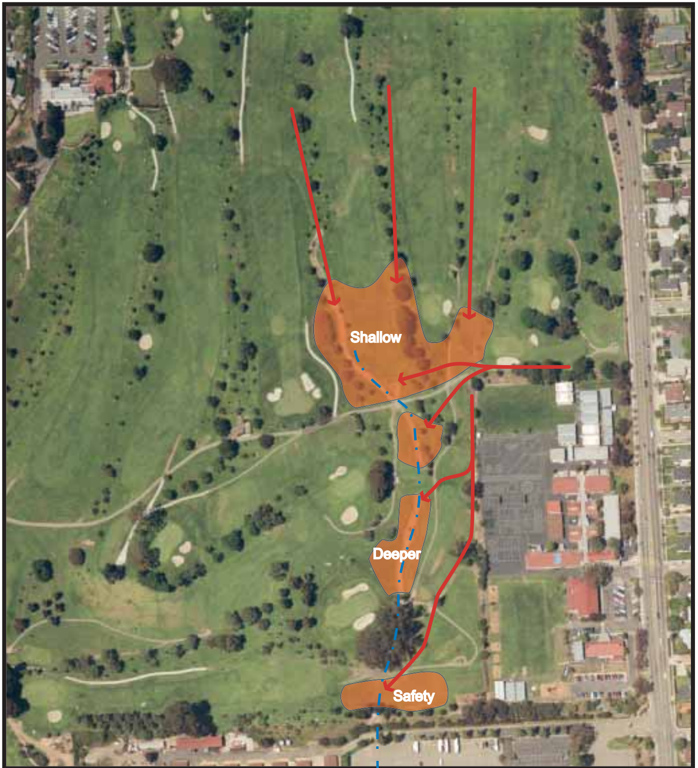
Dry Detention Pond Concept Santa Barbara Golf Course Bradley Owens, GeoSyntec Consultants
